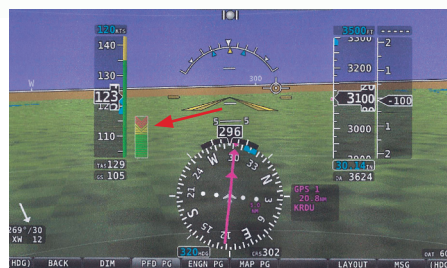
The latest Dynon SkyView EFIS with AOA display (marked by red arrow). In earlier versions the AOA was more prominent
