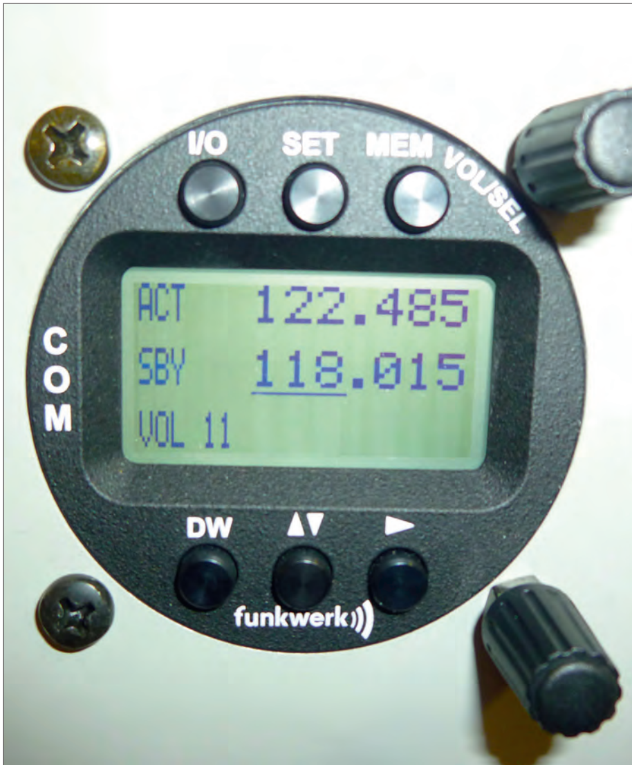
Funkwerk ATR833 radio with 8.33 channel selection
