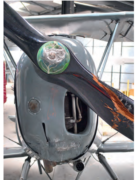
The damaged prop and 'gravel-rashed' nosebowl. Note cabbage paint scheme on crushed spinner.
