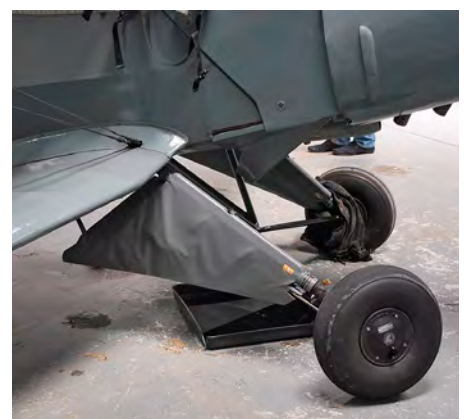
The offending starboard undercarriage leg that gave up in protest.
