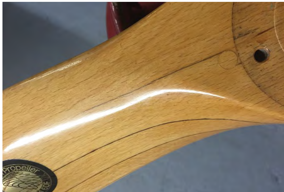
(Above) During a pre-flight inspection, LAA Inspector Matt Pettit noticed this deep crack emanating from the plugged balance weight on this Newton 54in propeller, as fitted to a Jodel D9. Records indicate that this propeller had completed about 400 hours and in all other respects appeared in first-class condition. Sadly, this propeller was effectively scrap, although I expect it will end up as a barometer mount affixed to a study wall. Well done to Matt for picking this up; remember that the pre-flight inspection is, from a pilot's perspective, most probably the most important inspection he or she will do, and it's certainly worth the extra effort required to do the job properly. (Photo: Matt Pettit)
