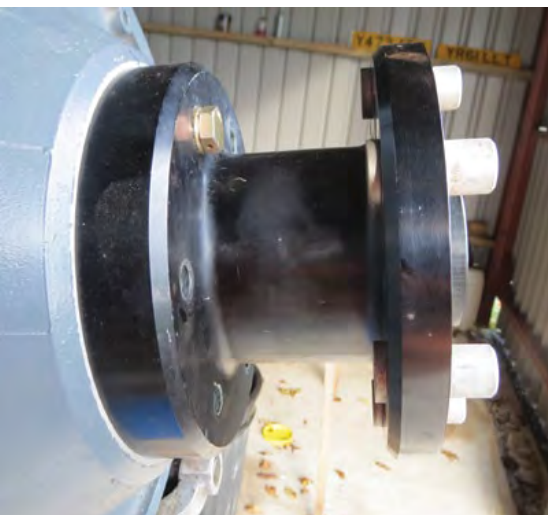
(Above) The propeller extension as fitted to Rob's RV-3 (to the left is the starter ring gear). The ferrules, colloquially called 'Top Hats', act as both a nut and to provide a positive location of the propeller. (Photo: Rob Hatwell)
