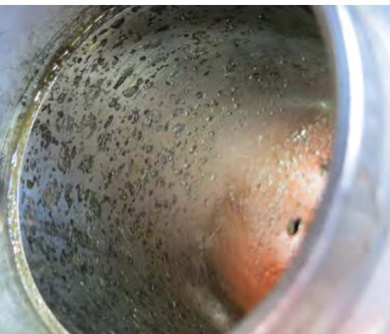
(Above) This picture shows the extent of the corrosion still remaining after cleaning and polishing the internal bore of the crankshaft on Rob Hatwell's RV-3 engine. Clearly, this crank isn't serviceable. (Photo: Rob Hatwell)
