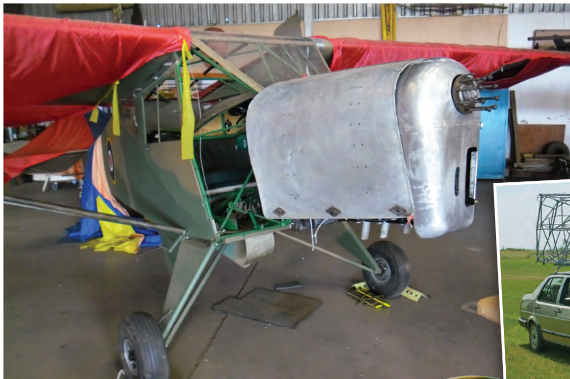
(Left) The scratch-made nose bowl, complete with wire edging as per the plans gratefully received from Peter Stoddart at Leicestershire Museum
