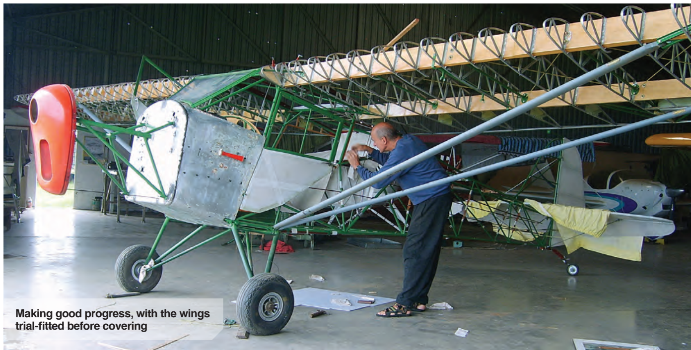
(Left) The scratch-made nose bowl, complete with wire edging as per the plans gratefully received from Peter Stoddart at Leicestershire Museum
