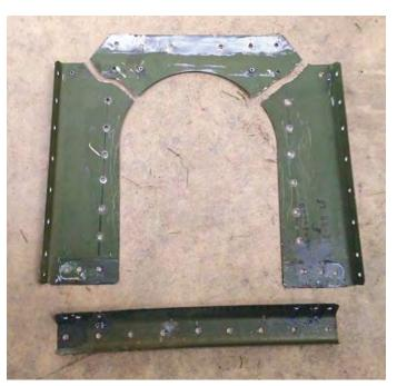
Though just a small crack could be seen during an initial close inspection, this is what was found when the frame was completely removed. As you can see, the structural integrity of the main connecting structure to the forward tailplane attachment has been completely lost. (Photo Chris Theakstone)
