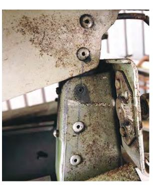
(Left) Here's a picture showing one tell-tale sign that all is not well with a riveted joint, notice the black powdery substance surrounding the third rivet up. This normally means that the rivet has become loose and therefore stopped working. This bracket, this time from the real tail attachment of a fairly high-time EV97, attaches the threaded steel plate holding the horizontal tail surfaces in place. (Photo Chris Theakstone)
