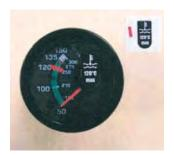
(Above and right) It is essential that a pilot is presented with appropriate and accurate information about the engines performance and, most importantly, its temperature relative to its operating maximums. We've come across examples in our fleet where a sender is measuring water temperature but the gauge fitted was marked-up as a CHT gauge.
