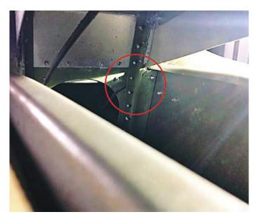
This picture shows the cracked bulkhead on a 4,000+ hrs EV97 training aircraft as spotted using a small camera. Certainly, boroscopes, cameras and even mobile phone technology can be very useful for looking into areas of a structure that have limited access. It's always better though to do a close visual inspection, if necessary by removing flight control surfaces, seats, panels, tanks or other assemblies, to gain access.
