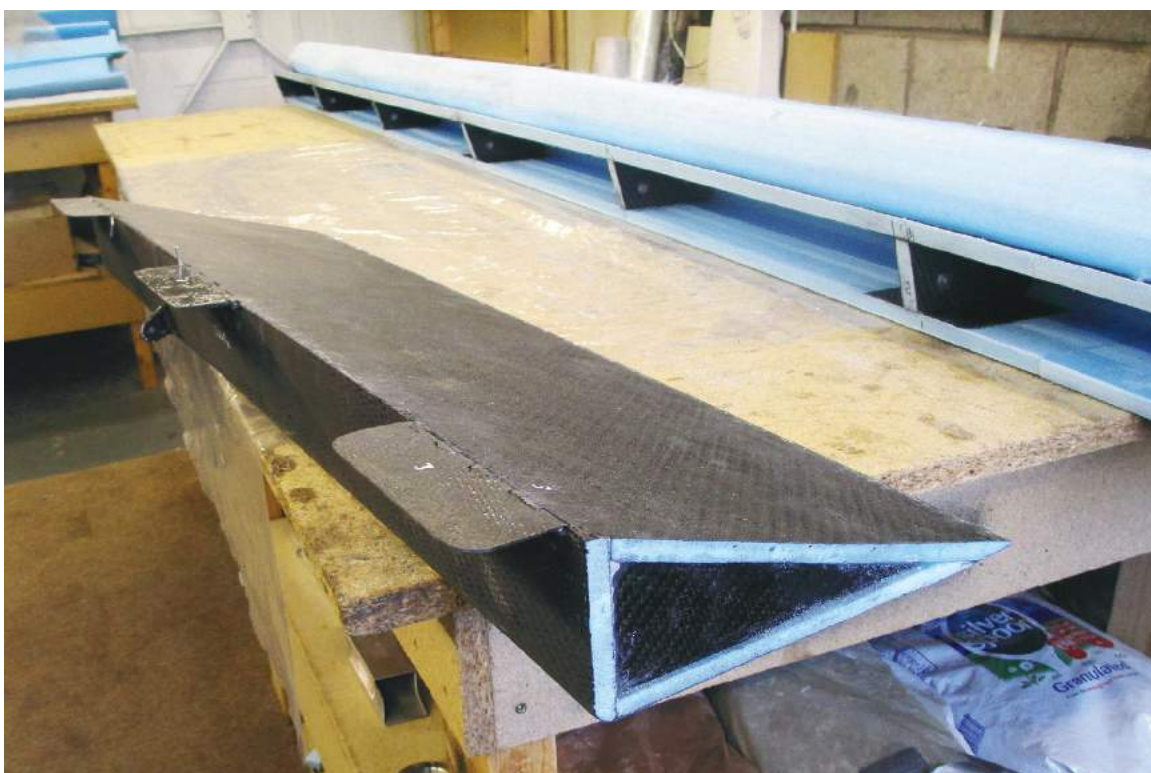
(Above) 9ft long flaps should help keep Blue 2 within the 35kt microlight stall speed limit.
