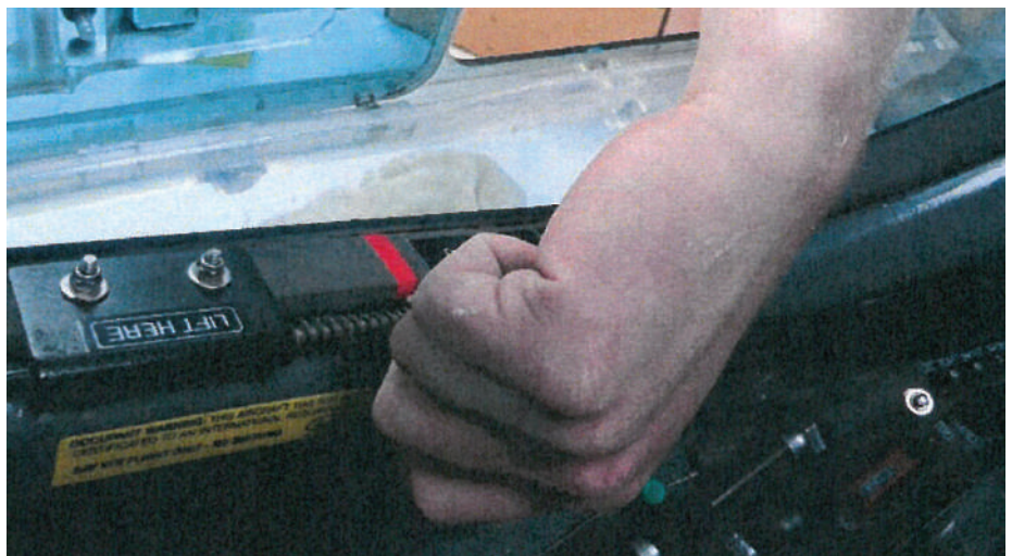
(Above) Although the method of getting into and out of an aircraft might seem obvious to the aviator, it'd be wrong to assume it's instinctive to non-flyers. I've taken this picture, originally supplied by LAA Inspector, Peter Wells, straight out of the AAIB Bulletin . If you've had any experience of gliding you will immediately recognise that, to lift the canopy, you must reach for the catch through the DV window. However, because there were no placards directing the first responders to this procedure, potentially valuable moments were lost during the pilot's rescue. (Photo: UK AAIB)
