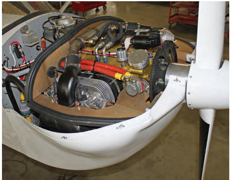
(Above) There are numerous VW aero-conversions in service today, some certified for aircraft use like the German Limbach and Sauer engines, and many operating in the world of the amateur-builder. The Sauer 2400UL engine is shown here neatly packaged into a Groppo Trail, a two-seat, high-wing kit-build. Note the position of the mechanical fuel pump and electronic ignition module (Starboard side/front). (Photo: Graham Smith)
