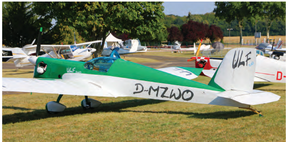
(Right) There were three of these Citroën Visa flat-twin car engine-powered EEL ULF 2s at Brienne. Designed in Germany by Dieter Reich, this ultralight motorglider first flew in 1993. It features a catalytic converter and a silencer which is reputed to reduce noise to 55db. The cruise speed is 75mph, its empty weight 210kg, the mauw 323kg and a ballistic chute can be installed behind the seat. The wingspan is eleven metres but they pull out from the fuselage and fold back. The tailplane is removable and, therefore, the ULF 2s can be transported by trailer. It’s of wood-and-fabric construction, and the plans, which include the details of the engine conversion, cost €350 and are available in German or English. www.eel.de/english/about.htm (Photo: Nigel Hitchman)
