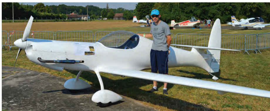
(Above) The Exia is a new, single-place prototype which will fall into the SDDR category in the UK. It was designed and built by Arnaud Abt (pictured) and first flew on 2 May this year. It's of all-composite construction and is powered by the Aixro XF40 wankel rotary engine, which puts out 35hp at 6,500rpm. Currently, the empty weight is 134kg but Arnaud is confident he can reduce that to 120kg so that it'll be eligible for the German 120kg class. The mauw is 220kg and it cruises at 95kt (175 kph). The plan is to put the design into kit production. (Photo: Brian Hope)
