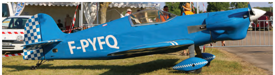
(Right) This is a nice example of a homebuilt French F1 racer from the seventies. It’s a Max Plan MP205, which is of wood-and-fabric construction and powered by a Continental O-200. (Photo: Nigel Hitchman)
