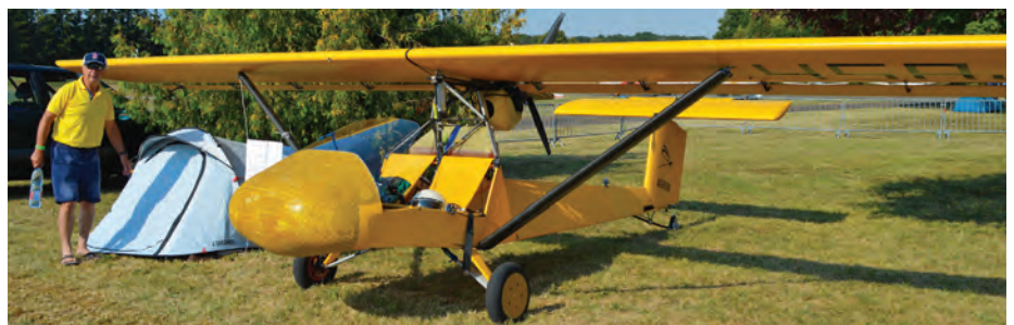
(Right) This two-seat Agrion microlight was badly damaged at last year’s RSA Rally, when it was blown across the airfield during a severe thunderstorm on the Saturday night. It’s an interesting machine as it features carbon-tube construction and weighs only 90kg empty. The mauw is 320kg and power comes courtesy of a 35hp Polini Thor 250. (Photo: Brian Hope)
