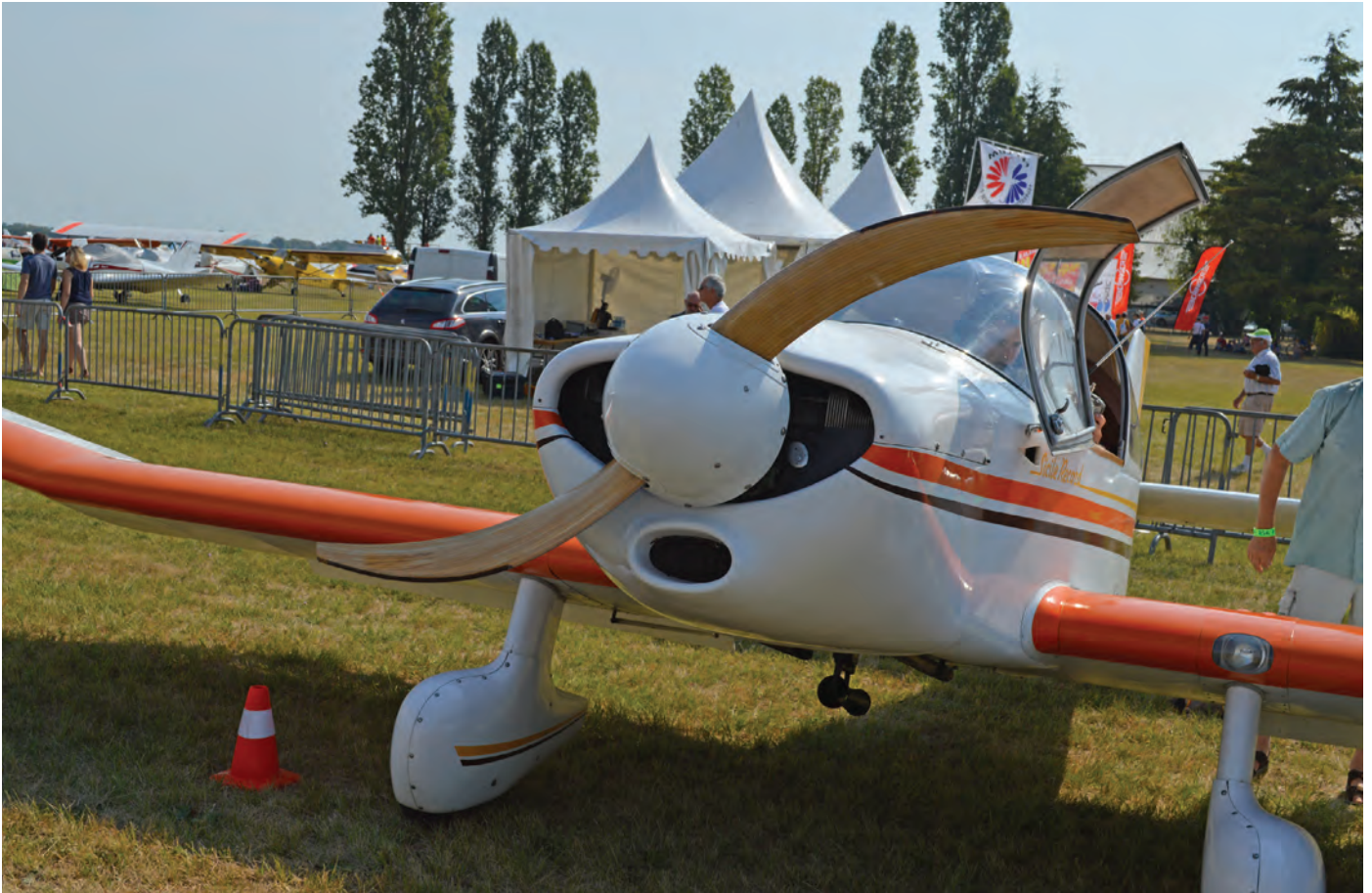
(Above) Wooden propellers, like this impressive scimitar example, seen recently on a French Jodel at the RSA Rally at Brienne-le-Château, are susceptible to dimensional shifts as their moisture content changes with the seasons. It's imperative that owners ensure the prop bolt torques are checked seasonally, to make sure that looseness (leading to potential departure!) or over-tightness (leading to crushing) doesn't occur. (Photo: Brian Hope)
