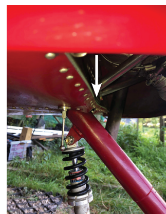
Above When Foxbat flyer, David Howell, carried out his pre-flight inspection, the first sign that all was not well with his aircraft was that the trailing edge of the propeller was clipping the engine cowling. Further investigation revealed the area of firewall and fuselage floor supporting the nose undercarriage attachment had buckled. David couldn't recall having suffered a heavier than normal landing – what on Earth could be going on? Photos: David Howell
