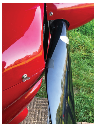
Above When Foxbat flyer, David Howell, carried out his pre-flight inspection, the first sign that all was not well with his aircraft was that the trailing edge of the propeller was clipping the engine cowling. Further investigation revealed the area of firewall and fuselage floor supporting the nose undercarriage attachment had buckled. David couldn't recall having suffered a heavier than normal landing – what on Earth could be going on? Photos: David Howell
