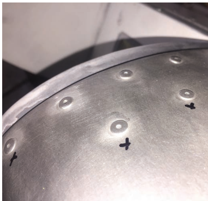
Above and right LAA Inspector, Nick Stone, came across a problem on a Bristell that was being prepared for respray recently, and got in touch. As you can see, especially when looking at the picture above, the Avex (pulled) rivets, have lost quite a bit of their head during the pre-primer preparation process. In a few cases, so much material has been lost that, in Nick's view, the aircraft's structure had been compromised. Both wings were returned to the aircraft's manufacturer for repair, an expensive exercise as quite a few rivets, and the fuel tanks, needed replacing. Happily, the wings have been returned to the owner and have been refitted to the fuselage. Photos: Nick Stone.
