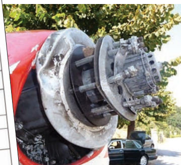
Left and above A recent DGAC AD requires owners of Stampe SV-4 aircraft to check the attachment of their propellers following a ditching incident, caused by a propeller detachment – in 2009. Note the failed Tab Washers behind the attachment nuts. Photos: DGAC/Mark Jeffries
