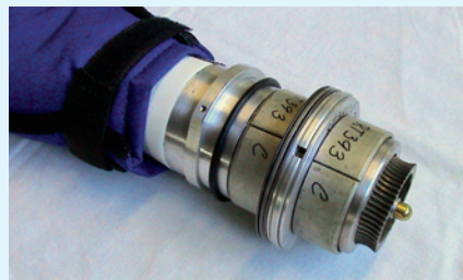
The SR 3000 blade at the root end disassembled from its hub
