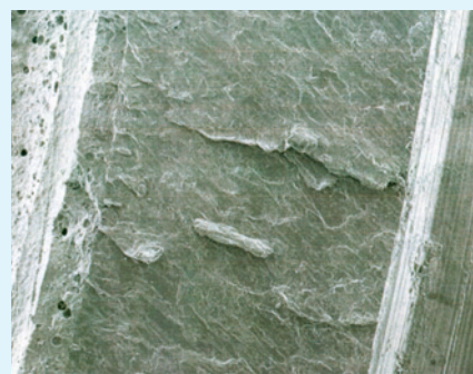
Micrograph showing delamination of the fracture surface
