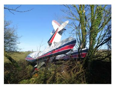
Fig 1. The Pilot of this Steen Skybolt recently suffered a catastrophic mechanical failure of his engine; the aircraft entered a spin and was brought to rest by a copse of trees. The pilot suffered only minor injuries and was able to walk clear of the aircraft because of a good deal of luck (a well-placed spinney) and a full harness that was in perfect condition.
