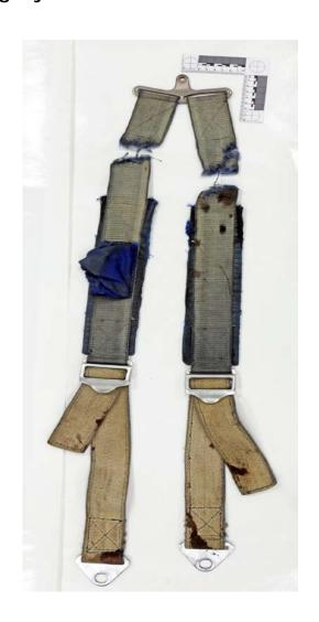
Fig 2. One pilot died and the other was seriously injured during an unsuccessful forced landing after an engine stoppage in a YAK-52 aircraft. The picture above shows the failed rear seat shoulder harness – when tested it was found that the harness had degraded such that its strength had reduced by up to 50%.
