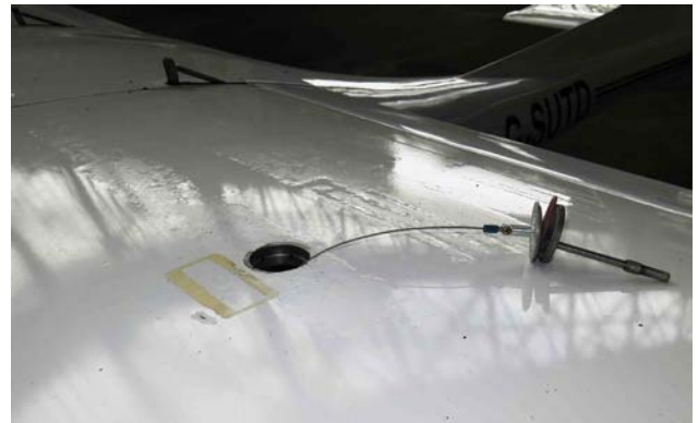
Fig 1. This picture shows the top surface of a Jabiru UL-D wing that's been affected by Mogas that's been left in the tank for some time. The UL-D is a factory built microlight and therefore considered a 'certified' type by the manufacturers and the UK CAA – it is therefore not approved automatically to use Mogas.
