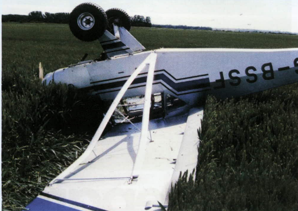
Looks bad, but the aircraft wasn't too badly damaged. Flip caused by standing crops, not the actual landing.
